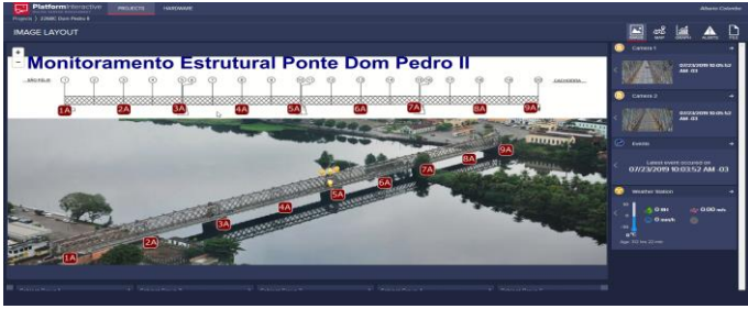
Figure 8. Dom Pedro II Bridge, a four span puddled iron truss bridge – Monitoring System using Cloud Computing.
